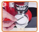
Put the circular pattern into the base mold
